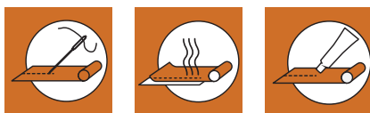
sewable, weldble & glueable | näh-, schweiß- & klebbar Glueing tested with Orafol Orabon 1397pp double-sided tape
